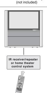
With this connection, point the Toshiba TV remote control at the front of the IR receiver/repeater or home theater control system to operate the TV.
